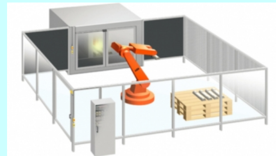
Traditional robot workcell setup
